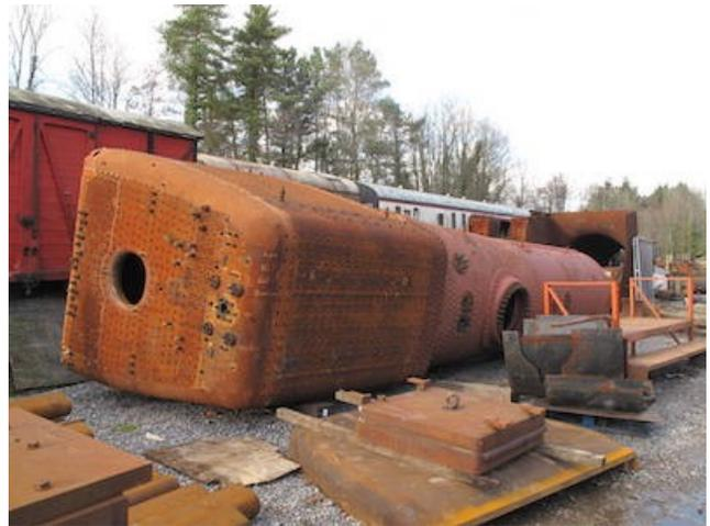
*Newly arrived at South Devon Railway, No. 34059's boiler awaits a survey. The boiler behind is from No. 34101 "Hartland".*
