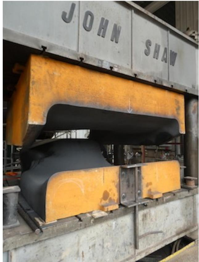
*Pressing of the combined combustion chamber and throat plate for No. 34059, using the 700-ton press at South Devon Railway, on 27 Sept., 2017*
