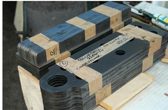
Sets of new liners for horn-guides and axle-boxes
