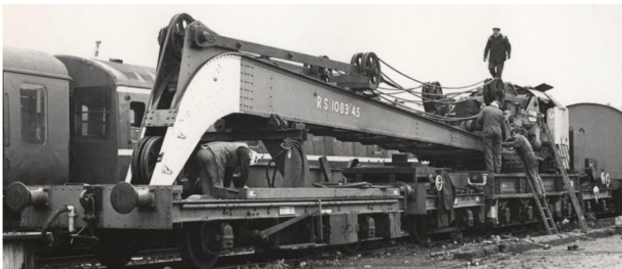
Hoist rope and jib ropes are removed from the jib, which will be craned off for separate movement, the jib runner and the jib travelled to Sussex in that order using the same flatbed lorry over 2 round trips.
